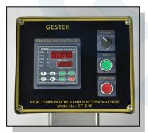
Power switch Start/Stop button Tem. Control gauge
