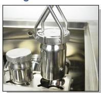
Use specified plug clamp the beaker, press and rotate to remove the beaker.
