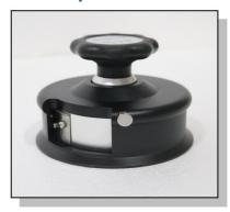
Pull it and rotate the side, cutter can be used.
