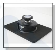
Circular sample cutter with cutting mat.
