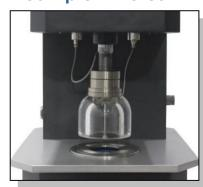
PMMA Cover, avoid to be hurt.make it's safety. Upper press plate inner dia.: 10cm2 Lower device test area: 7.3cm2
